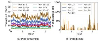
Figure 3: Load imbalance among equivalent upstream links of an Aggregation switch in production data center.
