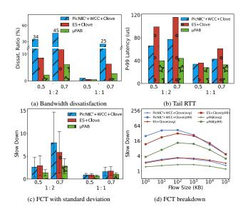
Figure 17: Performance under real workload with 1:2, 1:1 oversubscription network and loads of 0.5 and 0.7.
